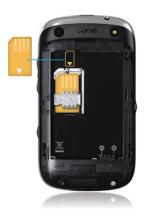
Slide the SIM card into the slot.
